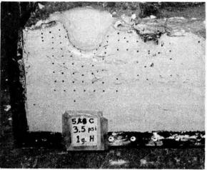
GEOTECHNICS—A one-gram explosive charge is detonated in an earth model accelerated to 100 g's on Sandia's centrifuge facility. At 100 g's, one gram of explosive is scalable to one ton. The resulting small crater is an accurate model of a larger event. Dark spots in the model are beads with which the kinetics of the cratering process can be recorded on high-speed motion picture film.
